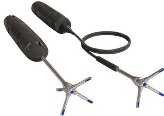
Figure-4 ADV with transducer and probes (Courtesy:Google)
