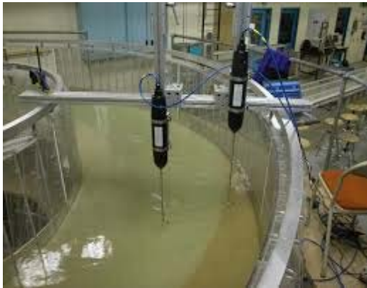
Figure -3 Real time application of ADV
