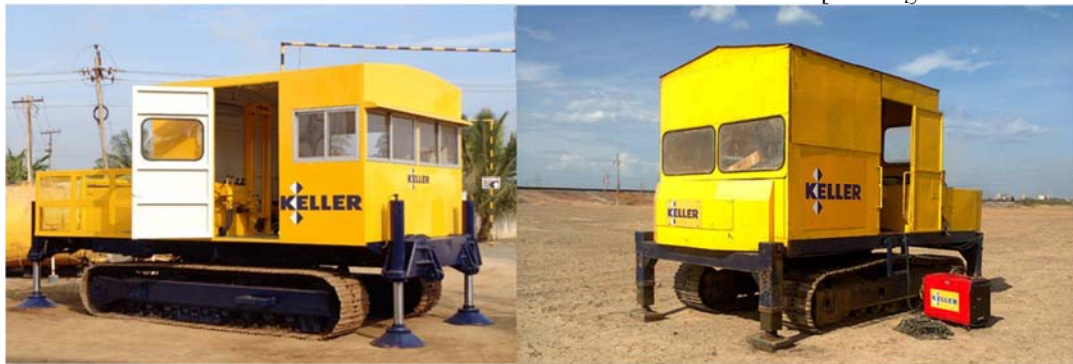
Figure 5: Electric Cone Penetration Testing Equipment
